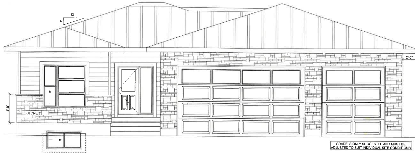
FRONT ELEVATION SCALE: 1/4" = 1'-0" 1x6 SMART TRIM AROUND ALL WINDOWS AND DOORS 1x6 SMART TRIM CORNER BOARDS
